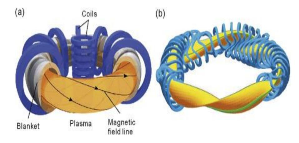
Schematics of magnetically confined plasmas in (a) tokamaks; (b) stellarator configurations. In the tokamak, the rotational transform of a helical magnetic field is formed by a toroidal field generated by external coils together with a poloidal field generated by the plasma current. In the stellarator, the twisting field is produced entirely by external non-axisymmetric coils.
