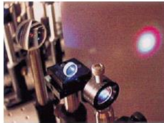
Figure 12 (a) Chirp on an ultrashort pulse induced by the nonlinear refractive index of a dielectric medium. The input pulse has a \text{sech}^2 envelope and the figure shows the instantaneous frequency within the pulse. A Taylor expansion around the peak of the pulse shows that the frequency sweep is approximately linear around time zero. (b) Photograph of a femtosecond white-light continuum beam generated in a piece of sapphire. (Picture courtesy of the Center for Ultrafast Optical Science, University of Michigan.)
